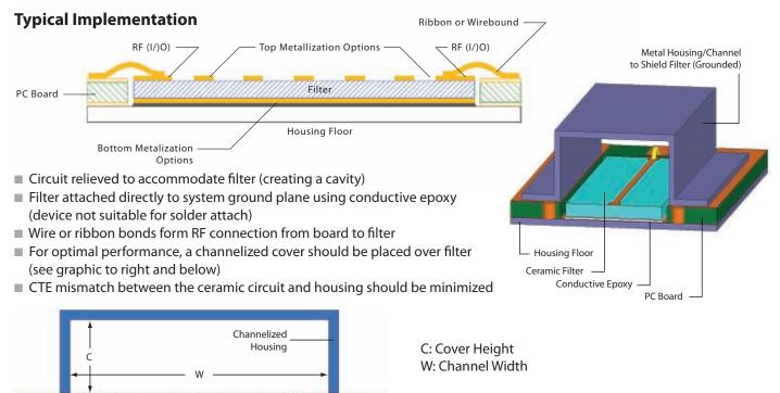
Customers can state a desired cover height and channel width or DLI engineering can make a recommendation based on the filter design
