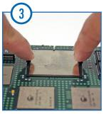
To ensure a secure fit, push spread apart FC slightly at the "horseshoe" tabs while pressing down.
