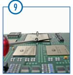
Remove the FC by placeing a small screwdriver within the "horseshoe" tab and gently twisting in either direction to pull the frame clip away from the component.
