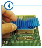
Place HS over the installed FC so that the "horseshoe" tabs of the FC fit within the HS' notches.
