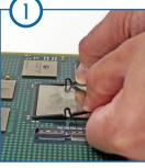
Place FC around two corners of the component. FC will bend slightly at the "horseshoe" tab. Note the direction of air flow when placing your HS.
