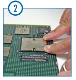
Press opposite end of the FC down until it is secure around the component's edges.
