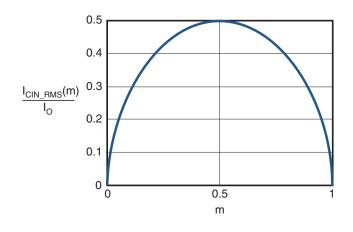
Figure 2. I<sub>CIN</sub> vs. Voltage Conversion Ratio
