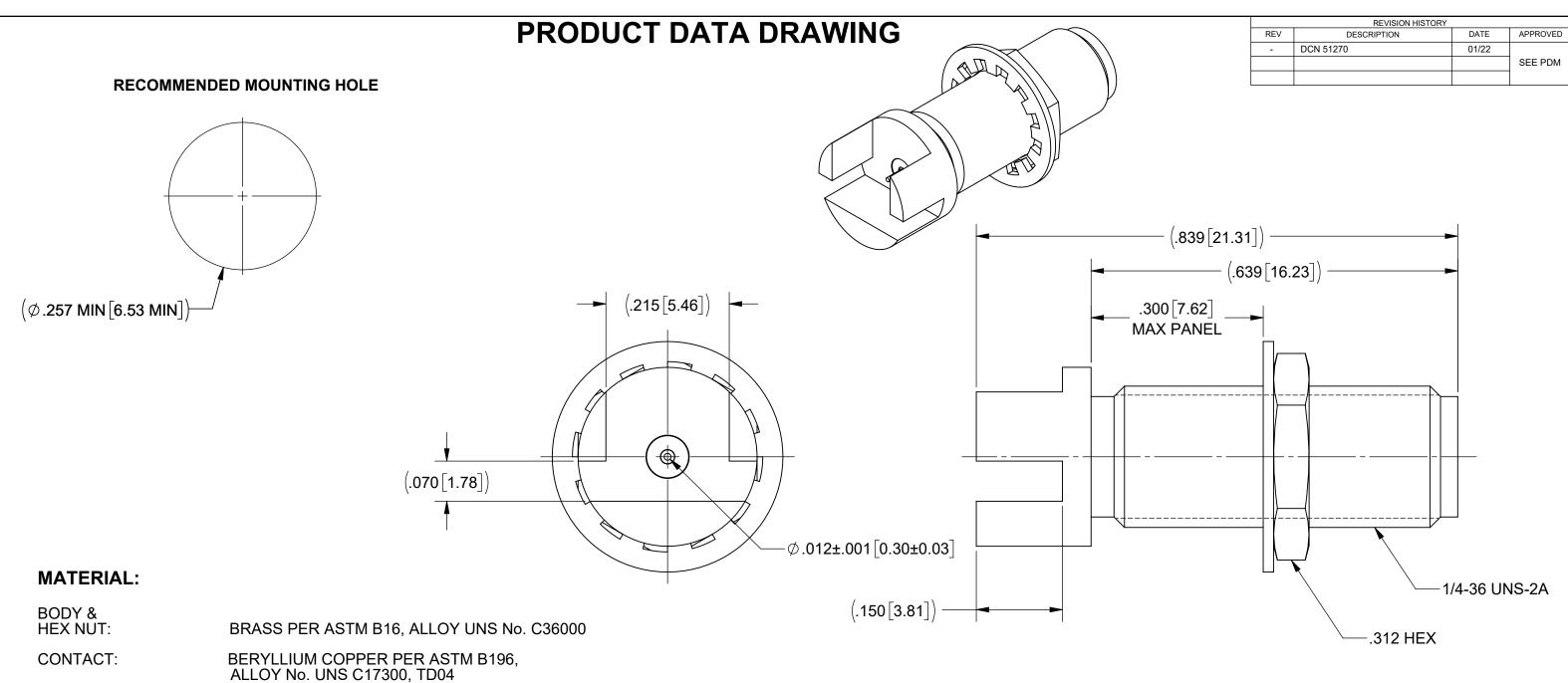
PTFE PER ASTM D1710, TYPE I, GRADE 1, CLASS B **INSULATOR:**
