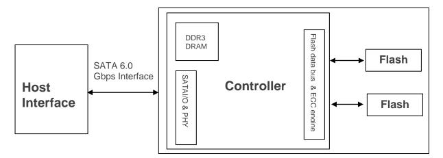
Figure 2-1 Block Diagram
