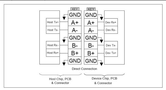
Figure 3-1 Direct Connection between the Host and Device
