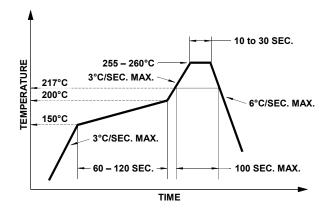
Figure 22: Recommended Board Reflow Direction
