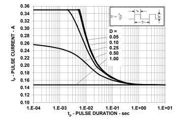
Figure 16: Pulse Handling Capability at T<sub>S</sub> ≤ 80°C
