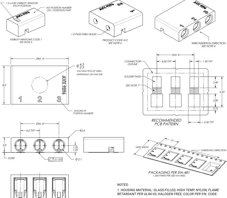
2. CONTACT MATERIAL: HIGH STRENGTH COPPER ALLOY;
