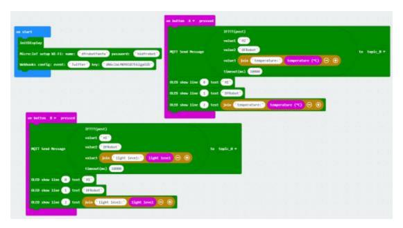
• Result: press down button A, send the message to Twitter: Hi DFROBOT and the current temperature; Press down button B, send: HI DFROBOT, and the current light intensity.
