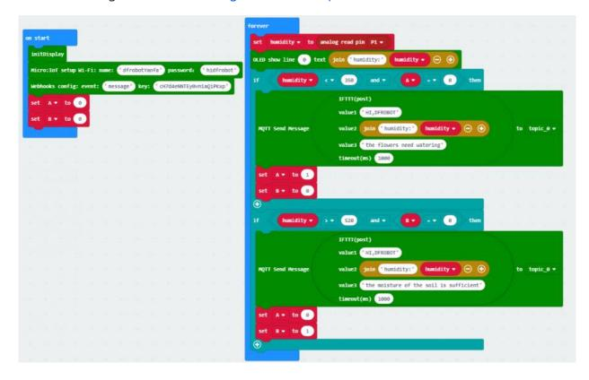
• Result: when moisture < 350, send: the flowers need watering; When moisture > 250, send: the moisture of the soil is sufficient.
