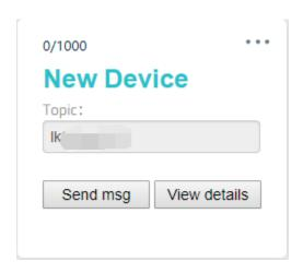
• Input your command into the blank, and send it out. Send the message "yes", micro:bit displays "√"; "no", "×"; "cry", "crying face pattern"; "smile", "smiley face".
