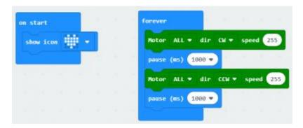
Result: the motor rotates forward at speed of 255 for 1 second, and then rotate backward for 1 second.
