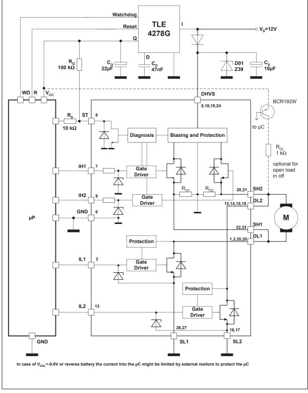
Figure 4 Application Circuit
