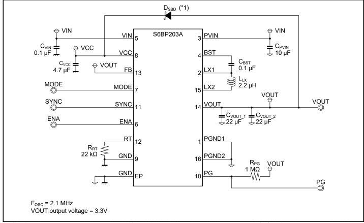
\*1: The D<sub>SBD</sub> is necessary only when using at VIN  $\leq$  3.3V. In addition, since a leakage current (I<sub>R</sub>) of the D<sub>SBD</sub> increases under high temperature, it is necessary to connect a load according to the leakage current of the D<sub>SBD</sub> to VOUT pin under the automatic PWM/PFM switching operation (MODE = L, SYNC = L).
