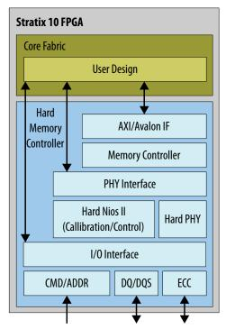
Each I/O bank contains 48 general purpose I/Os and a high-efficiency hard memory controller capable of supporting many different memory types, each with different performance capabilities. The hard memory controller is also capable of being bypassed and replaced by a soft controller implemented in user logic. The I/Os each have a hardened double data rate (DDR) read/write path (PHY) capable of performing key memory interface functionality such as:
