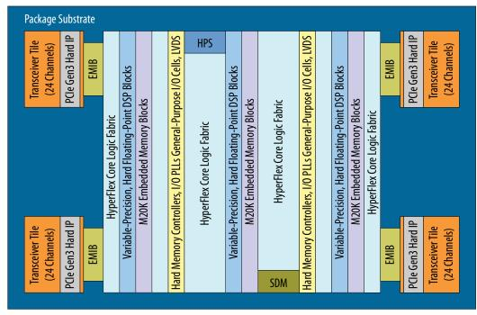
HPS: Quad ARM Cortex-A53 Hard Processor System
