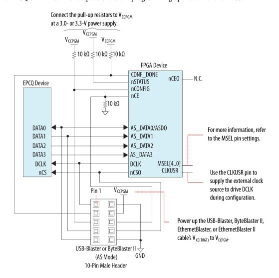
When programming the EPCS and EPCQ devices, the download cable disables access to the AS interface by driving the nCE pin high. The nCONFIG line is also pulled low to hold the Cyclone V device in the reset stage. After programming completes, the download cable releases nCE and nCONFIG, allowing the pull-down and pull-up resistors to drive the pin to GND and  $V_{CCPGM}$ , respectively.
