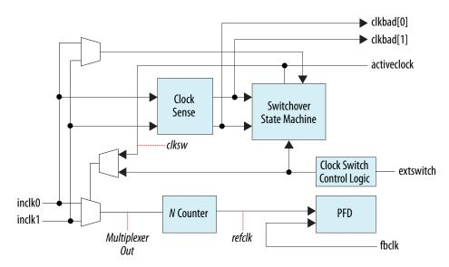
When the current reference clock is not present, the clock sense block automatically switches to the backup clock for PLL reference. You can select a clock source as the backup clock by connecting it to the inclk1 port of the PLL in your design.
