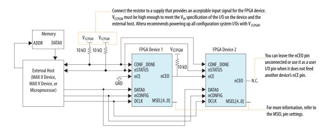
After a device completes configuration, its nCEO pin is released low to activate the nCE pin of the next device in the chain. Configuration automatically begins for the second device in one clock cycle.
