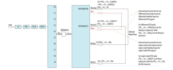
Figure 4-32: Example of Phase Relationship Between the PLL Clocks in EFB Mode
