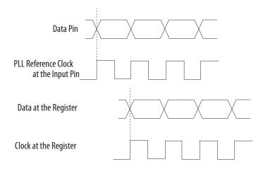
The source synchronous mode compensates for the delay of the clock network used and any difference in the delay between the following two paths:
