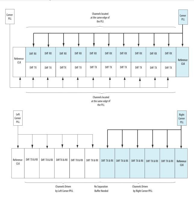
Figure 5-3: Invalid Placement of Differential I/Os Due to Interleaving of Channels Driven by the Corner PLLs
