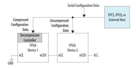
For the FPP configuration scheme, a combination of compressed and uncompressed configuration in the same multi-device configuration chain is not allowed because of the difference on the DCLK-to-DATA[] ratio.
