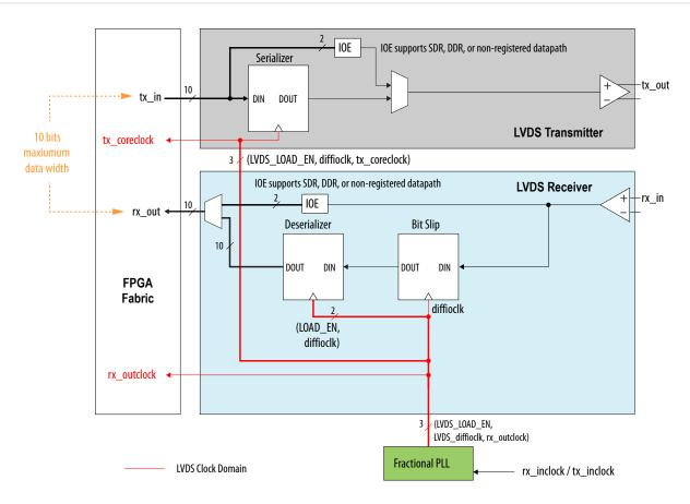
The preceding figure shows a shared PLL between the transmitter and receiver. If the transmitter and receiver do not share the same PLL, you require two fractional PLLs. In single data rate (SDR) and double data rate (DDR) modes, the data width is 1 and 2 bits, respectively.
