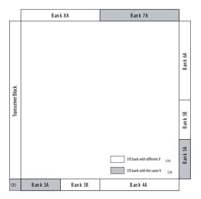
Because banks 5A and 7A have the same  $V_{CCIO}$  as bank 3A, you can calibrate all three I/O banks (3A, 5A, and 7A) with the OCT calibration block (CB3) located in bank 3A.
