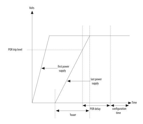
The Cyclone V POR circuitry uses an individual detecting circuitry to monitor each of the configuration-related power supplies independently. The main POR circuitry is gated by the outputs of all the individual detectors. The main POR signal is asserted when the power starts to ramp up. This signal is released after the last ramp-up power reaches the POR trip level during power up.
