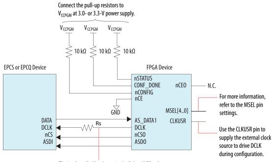
This is only applicable when using the Cyclone V QS package. For more information, refer to section 1.6 of AN822.
