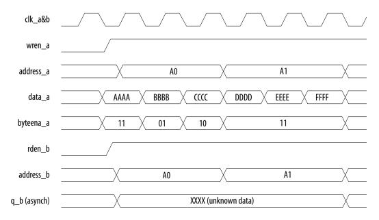
In the dual-port RAM mode, the mixed-port read-during-write operation is supported if the input registers have the same clock. The output value during the operation is "unknown."
