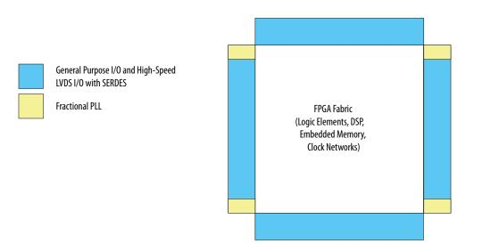
Figure 5-30: High-Speed Differential I/O Locations in Cyclone V GX C3 Devices
