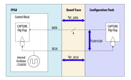
The data setup timing slack must be equal or larger than the minimum data setup time, t<sub>DSU</sub>
