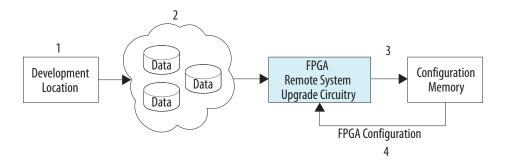
You can design your system to manage remote upgrades of the application configuration images in the configuration device. The following list is the sequence of the remote system upgrade:
