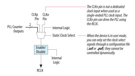
You can set the input clock sources and the clkena signals for the GCLK and RCLK network multiplexers through the Intel Quartus Prime software using the ALTCLKCTRL IP core.
