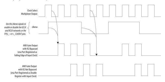
Cyclone V devices have an additional metastability register that aids in asynchronous enable and disable of the GCLK and RCLK networks. You can optionally bypass this register in the Intel Quartus Prime software.
