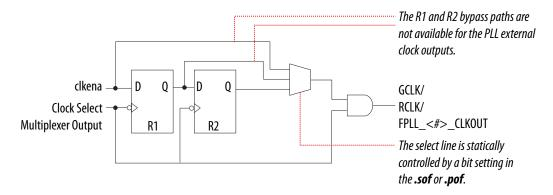
The clkena signals are supported at the clock network level instead of at the PLL output counter level. This allows you to gate off the clock even when you are not using a PLL. You can also use the clkena signals to control the dedicated external clocks from the PLLs.
