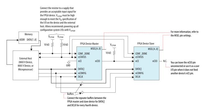
When a device completes configuration, its nCEO pin is released low to activate the nCE pin of the next device in the chain. Configuration automatically begins for the second device in one clock cycle.
