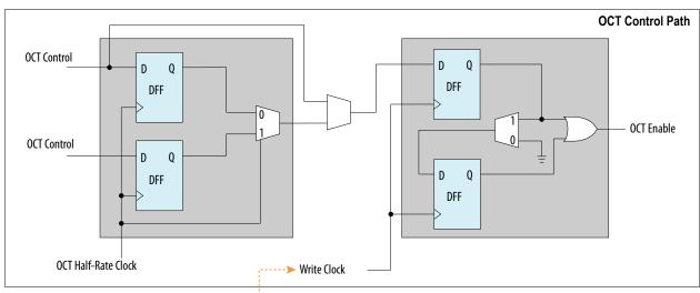
The full-rate write clock comes from the PLL. The DQ write clock and DQS write clock have a 90° offset between them
