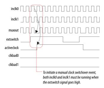
In automatic override with manual switchover mode, the activeclock signal mirrors the extswitch signal. Since both clocks are still functional during the manual switch, neither clkbad signal goes high. Because the switchover circuit is positive-edge sensitive, the falling edge of the extswitch signal does not cause the circuit to switch back from inclk1 to inclk0. When the extswitch signal goes high again, the process repeats.
