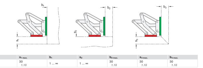
2. Mounting flange mounted to the housing with slotted holes perpendicular to the hinge axis:
