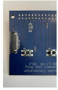
Figure 4: Closed Flex Connector
