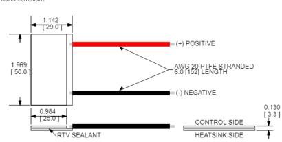
CERAMIC MATERIAL: Al<sub>2</sub>O<sub>3</sub> SOLDER CONSTRUCTION: 232°C, SbSn
