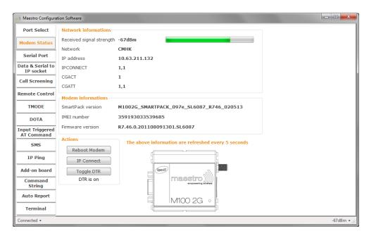
Figure 4.2.2: Status page - Maestro Configuration Software
