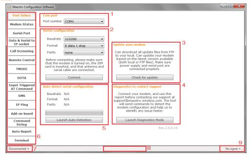
Figure 4.2.1: Start page - Maestro Configuration Software
