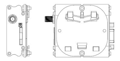
Figure 3.1.1: DIN clip mounted on M100 2G
