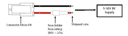
Figure 3.5.1: Power cord not included in the package
