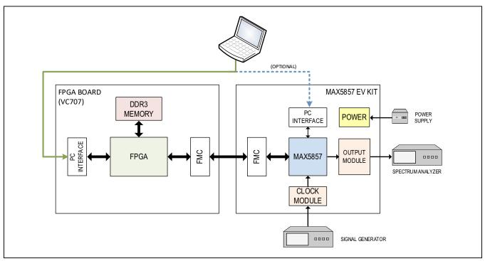
Figure 9. MAX5857 Evaluation System Block Diagram
