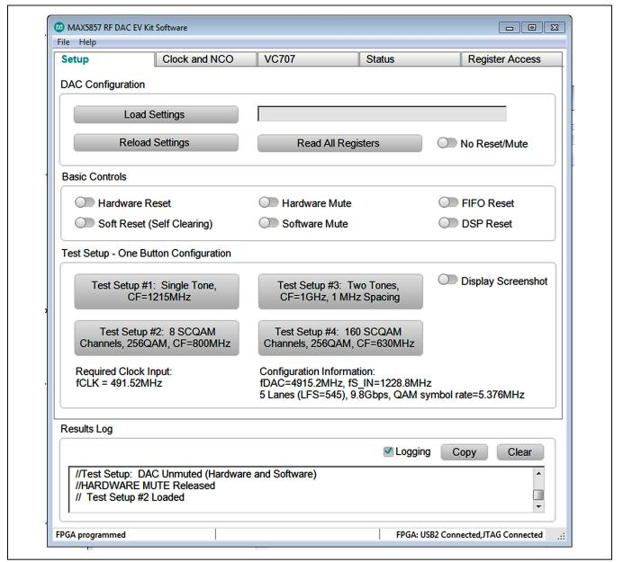
Figure 16. MAX5857 EV Kit GUI - Setup
