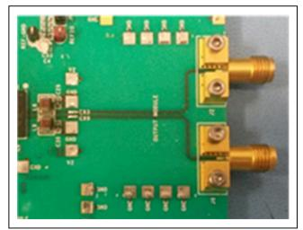
Figure 12. MAX5857 Differential DAC Output
