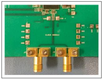
Figure 11. MAX5857 Differential Clock Input
