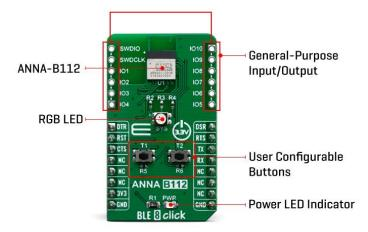
By integrating most of the critical components on the chip, the ANNA-B112 allows the module to overcome any imperfections of external discrete components, allowing signal transmission power of up to 5dBm, and -92 dBm sensitivity for the receiver, using the on-chip antenna.
