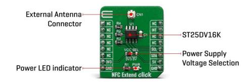
Depending on the application requirements various shapes and sizes of 13.56 MHz external antenna can be used by connecting them to CN1 (male U.FL) connector. Mikroe is working on offering plenty of them it in the future, therefore stay tuned.
