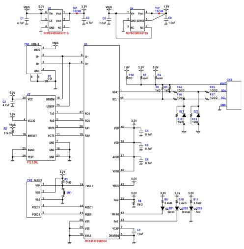
Figure 4. Interface Box Schematic
