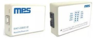
Figure 10: MPS EVKT-USBI2C-02 Communication Interface
