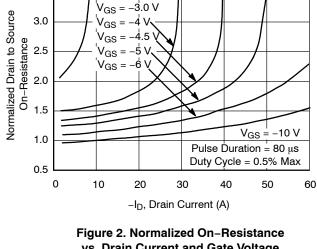
vs. Drain Current and Gate Voltage
