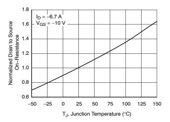
Figure 3. Normalized On-Resistance vs. Junction **Temperature**
