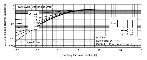
Figure 13. Transient Thermal Response Curve
