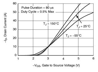
Figure 5. Transfer Characteristics
