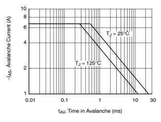
Figure 9. Unclamped Inductive Switching Capability
