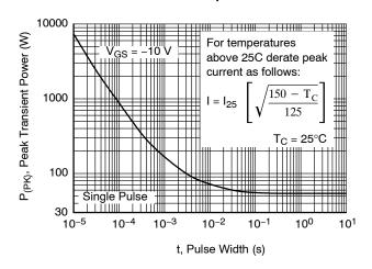
Figure 12. Single Pulse Maximum Power Dissipation
