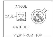
>Soldering Conditions: 260°C 1/16 inch away from case for 3 seconds max.
