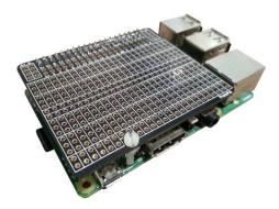
The ProtoPal is an affordable prototyping board for the Raspberry Pi 2, A+ and B+
