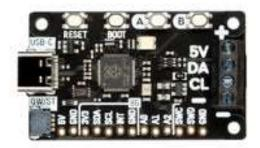
Swathe everything in rainbows with this all-in-one, USB-C powered controller for WS2812/Neopixel and APA102/Dotstar addressable LED strip.
