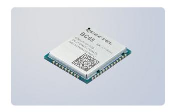
BC65 is high-performance multi-band NB-IoT module with extremely low power consumption. The ultra-compact 17.7mm × 15.8mm × 2.2mm profile makes it a perfect choice for size sensitive applications. Designed to be compatible with Quectel GSM/GPRS M66 , NB-IoT BC66 and BC68 modules in the compact and unified form factor, BC65 provides a flexible and scalable platform for migrating from GSM/GPRS to NB-IoT network.
