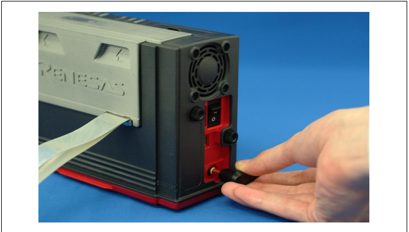
Figure 2.5 Connecting the emulator power supply
