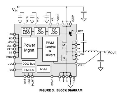
$<sup>^{\</sup>dagger}$  The DDC bus pull-up resistance will vary based on the capacitive loading of the bus, including the number of devices connected. The 10 k $\Omega$  default value, assuming a maximum of 100 pF per device, provides the necessary 1  $\mu$ s pull-up rise time. Please refer to the Digital-DC Bus section for more details.
