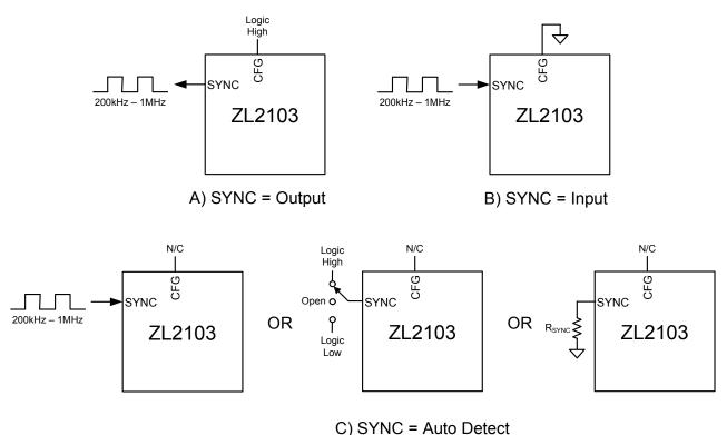
FIGURE 15. SYNC PIN CONFIGURATIONS
