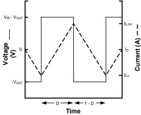
FIGURE 11. INDUCTOR WAVEFORM
