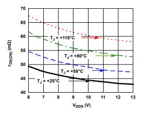
FIGURE 7. LOW-SIDE  $r_{DS(ON)}$  vs  $V_{DDS}$  WITH  $T_J$
