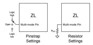
FIGURE 12. PIN-STRAP AND RESISTOR SETTING EXAMPLES
