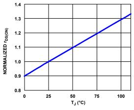
FIGURE 6. HIGH-SIDE  $r_{DS(0N)}$  vs  $T_J$  NORMALIZED FOR  $T_J = +25\,^{\circ}$  C ( $V_{DDS} = 12V$ , BST - SW = 6.5V,  $I_{DRAIN} = 0.3A$ )
