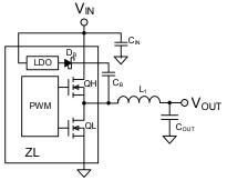
FIGURE 9. SYNCHRONOUS BUCK CONVERTER
