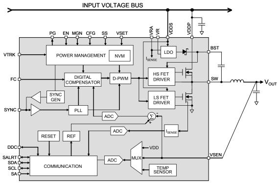
FIGURE 10. ZL2103 BLOCK DIAGRAM
