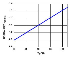
FIGURE 5. LOW-SIDE  $r_{DS(ON)}$  vs  $T_J$  NORMALIZED FOR  $T_J = +25$ °C ( $V_{DDS} = 12V$ ,  $I_{DRAIN} = 0.3A$ )
