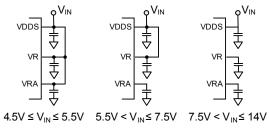
FIGURE 13. INPUT SUPPLY CONNECTIONS
