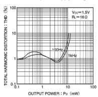
Fig. 17 Total harmonic distortion vs. output voltage
