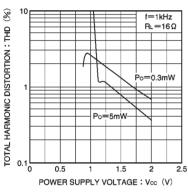
Fig. 16 Total harmonic distortion vs. power supply voltage
