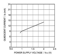
Fig. 10 Quiescent current vs. power supply voltage
