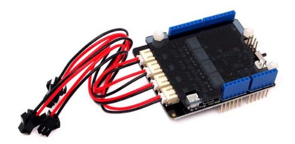
This shield is used to control EL devices. It can control 4 EL devices simultaneously. The controlling method is as simple as controlling an LED. Driven by PWM, it can create a colorful and florid effect by controlling each EL wire with a simple program. Combined with our EL Inverter, it can drive an EL wire as long as 15m, which provides infinite possibility for your design. Besides, the Shield is covered by Acrylic board, which enhances user's safety.
