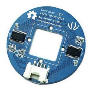
This is a unique ring—it has a florid body with 24 controllable LEDs. Maybe it will drive the inspiration out of you to make a glowing magic ring! There is a 1\*1 square hollowout in the middle of this module, where you can place a Grove Encoder in and make it a rotary visual encoder!
