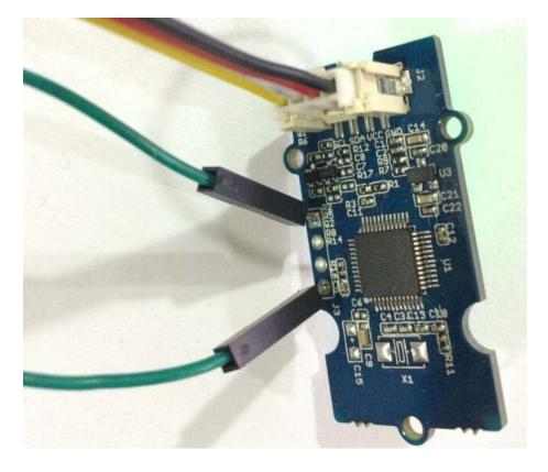
Interface: UART (the Grove connector supports I2C and UART), when upgrade the firmware, the Grove interface run in UART mode.
