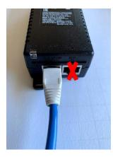
*Figure 7: Ethernet cable connected to the power brick*
