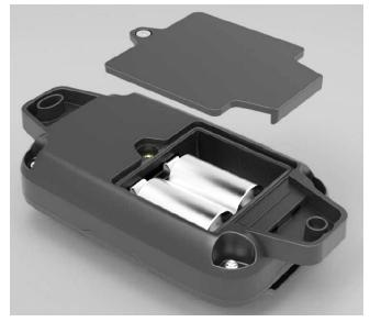
Figure 18: Changing sensor batteries
