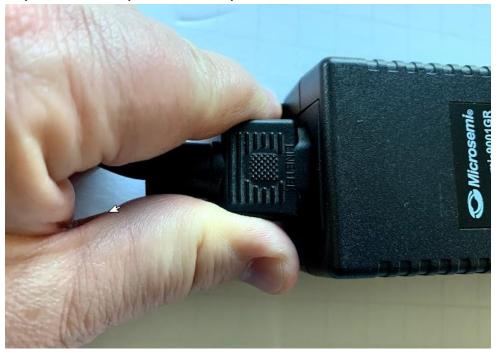
Step 8: Connect the power brick to a power source.
