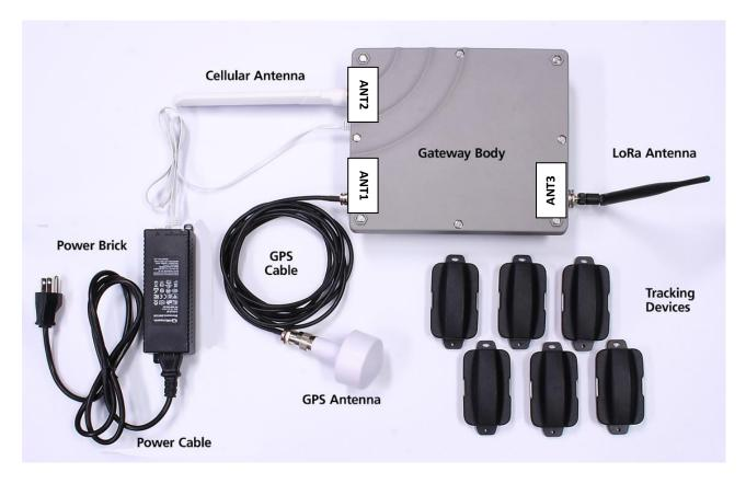
Figure 2: LoRaWAN gateway with 3G/4G LTE (Cellular) backhaul
