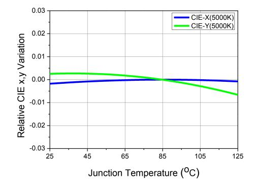
Fig 7. Junction Temperature vs. CIE x,y Shift, I<sub>F</sub>=0.43A (5000K)
