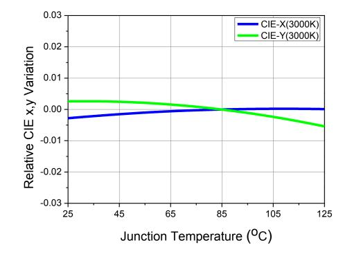
Fig 9. Junction Temperature vs. CIE x,y Shift, I<sub>F</sub>=0.43A (3000K)
