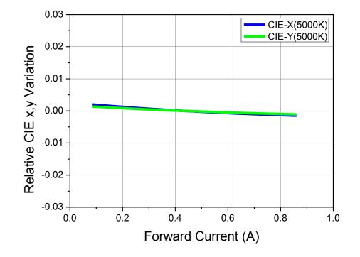
Fig 10. Forward Current vs. CIE x,y Shift, T<sub>j</sub>=85°C (5000K)
