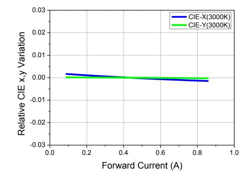
Fig 12. Forward Current vs. CIE x,y Shift, T<sub>j</sub>=85°C (3000K)
