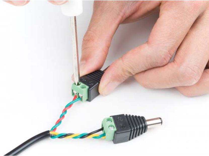
**Note:** Using screw terminals is one method of modifying the 12V/5V power supply. For a more secure connection, try splicing the wires to a polarized connector and adding heat shrink to your connection. You can also use a USB connector for the 5V side depending on your personal preferences.
