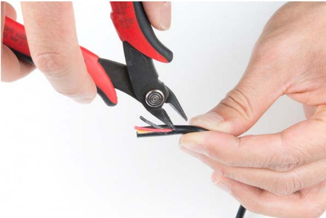
Strip the power supply's three wires. The wires are stranded so feel free to tin the wires by adding solder to the tips.
