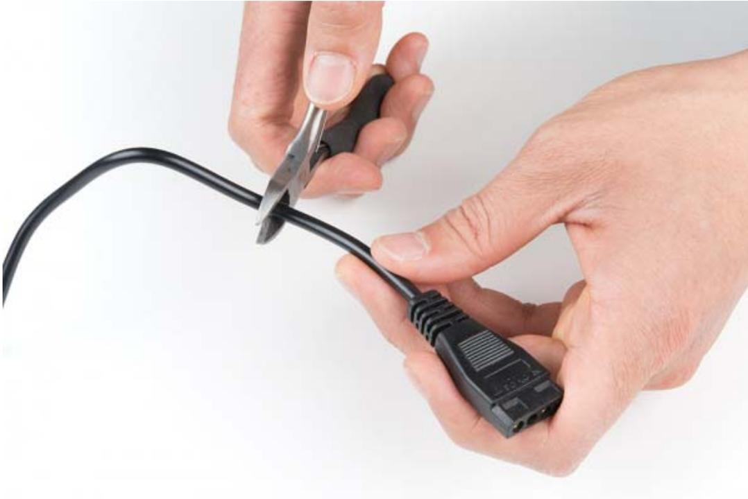
Cut into sheath with the flush cutter. Pull it back just enough so that you have enough room to work with the wires. Be careful not to cut yourself!
