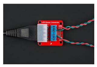
**Heads up!** If you are using only one of the voltages from the 12V/5V power supply, the other side may become unstable if there is not a minimum load (10mA) just like the note in the ATX power supply above. Depending on your project, you may need to add load in order for the voltage to become stable for long term installations. When testing it out with a multimeter without a load on both sides, the voltages appeared to be stable.
