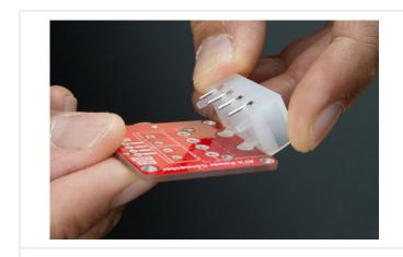
Insert Support Leg into Breakout
