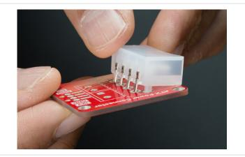
Sliding Pins into Breakout
