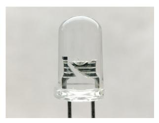
LED with Built-In Resistor Close Up
