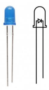
The positive side of the LED is called the "anode" and is marked by having a longer "lead," or leg. The other, negative side of the LED is called the "cathode." Current flows from the anode to the cathode and never the opposite direction. A reversed LED can keep an entire circuit from operating properly by blocking current flow. So don't freak out if adding an LED breaks your circuit. Try flipping it around.
