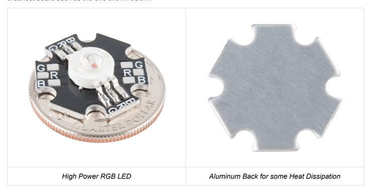
High-Power LEDs can generate so much waste heat that they'll damage themselves without proper cooling. Don't let the term "waste heat" fool you, though, these devices are still incredibly efficient compared to conventional bulbs. To control, you could use a constant current LED driver.
