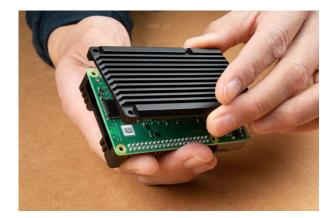
Screw and tighten the hex bolts using the allen key.
