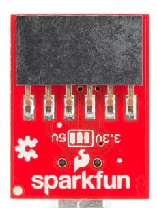
6 pin SIL, 0.1" pitch header at top of PCBA
