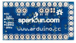
A4 and A5's location may be very important if you plan on using  $I^2C$  with the Pro Mini -- those are the hardware SDA and SCL pins.
