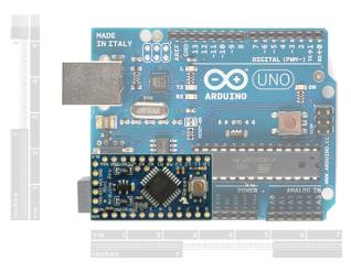
Comparing the size of a standard Arduino Uno with the (aptly named) Pro Mini.
