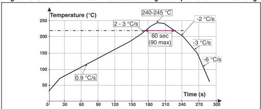
Note: Minimize air convection currents in the reflow oven to avoid component movement.
