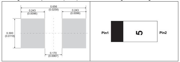
Note: The marking codes can be rotated by 90° or 180° to differentiate assembly location. In no case should this product marking be used to orient the component for its placement on a PCB. Only pin 1 mark is to be used for this purpose.
