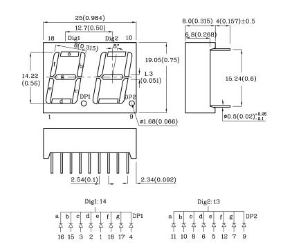
1. All dimensions are in millimeters (inches), Tolerance is  $\pm 0.25 (0.01")$  unless otherwise noted.
