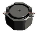
TAIYO YUDEN'S EST1040 series inductor is the latest in TAIYO YUDEN'S line up of EST series AEC-Q200 qualified grade 1 fixed inductors with a footprint of 10.0 x 10.0 x 4.3 mm. Available in inductance up to 470uH and tolerances of 20% and 30%. This fixed inductor is ideal for automotive and industrial
