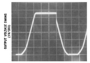
TIME (5  $\mu$ s/DIV) Figure 27. Current Limit (R<sub>L</sub>=100 $\Omega$ )
