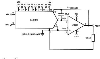
$$\begin{split} V_{OUT} &= -V_{REF} \left( \frac{A1}{2} + \frac{A2}{4} + \frac{A3}{8} + \frac{A10}{1024} \right) \\ &- 10V \leq V_{REF} \leq 10V \\ 0 \leq V_{OUT} \leq -\frac{1023}{1024} V_{REF} \end{split}$$
