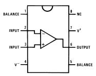
Figure 1. 8LD Ceramic Dual-in Line Package See Package Number NAB0008A (Top View)
