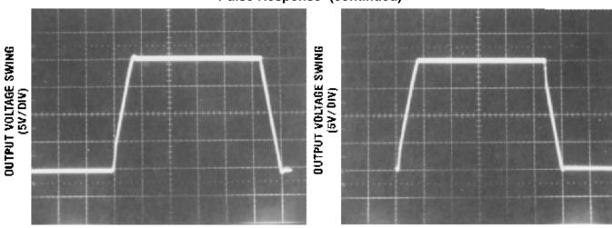
TIME (2 µs/DIV) Figure 25. Large Signal Inverting
