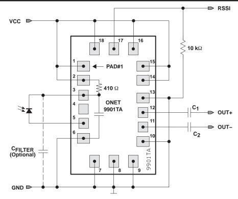
Figure 3. Basic Application Circuit
