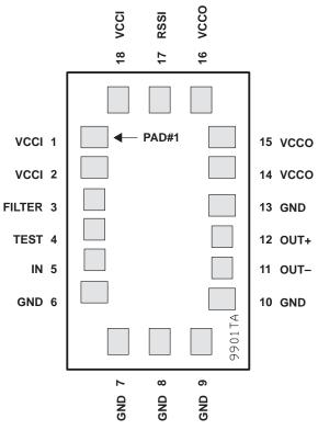
Figure 2. Bond Pad Assignment of the ONET9901TA
