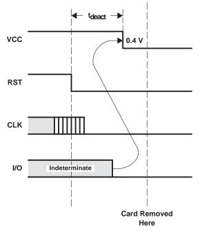
Figure 12–4. Contact Deactivation Sequence
