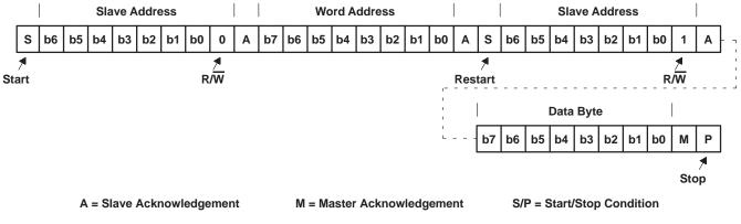
Figure 3–9. Serial-Bus Protocol—Byte Read
