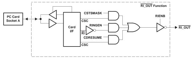
Figure 3–14. RI\_OUT Functional Diagram
