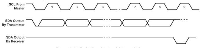
Figure 3–7. Serial-Bus Protocol Acknowledge
