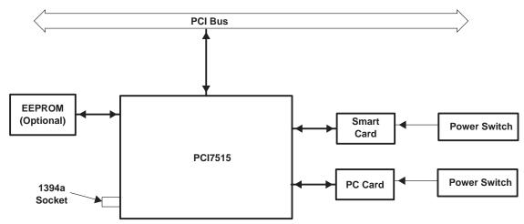
Figure 3–1. PCI7515 System Block Diagram
