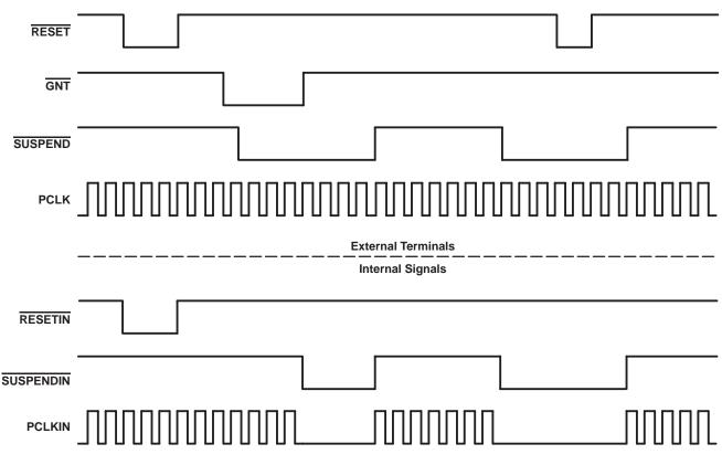
Figure 3–13. Signal Diagram of Suspend Function
