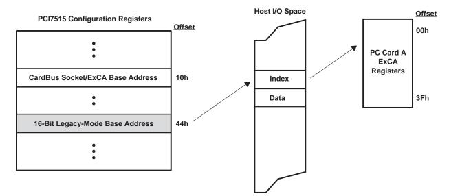
Offset of desired register is placed in the index register and the data from that location is returned in the data register.
