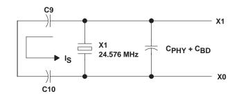
Figure 3–19. Load Capacitance for the PCI7515 PHY
