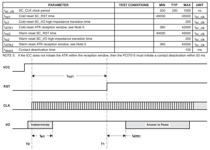
12.9 Smart Card Timing Specifications Over Recommended Operating Conditions
