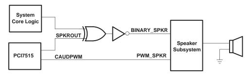
Figure 3–4. SPKROUT Connection to Speaker Driver
