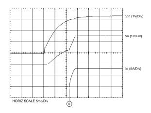
Figure 2-1; Schematic Demonstrating Startup into Pre-Bias Capability
