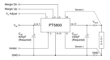
$C_{in}$  = Required 820µF  $C_{out}$  = Required 330µF
