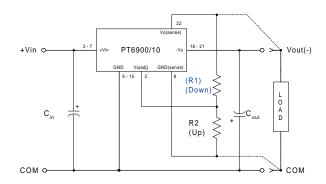
The respective values of (R1) [adjust down], and R2 [adjust up], can also be calculated using the following formulas.
