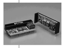
The PT7700 is a new series of highperformance, 15 Amp Integrated Switching Regulators (ISRs) housed in a 27-pin SIP package. The 15A capability allows easy integration of the latest high-speed, lowvoltage μPs and bus drivers into existing 5V systems.
