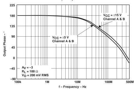
Figure 1–6. THS6062 EVM Phase vs. Frequency with Gain = -3
