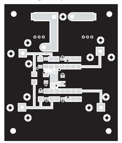
Figure 2–3. THS6062 EVM PC Board Layout – Component Side
