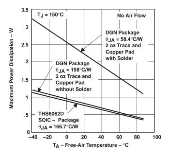
Even though the THS6062 EVM PCB is smaller than the one in the example above, the results should give an idea of how much power can be dissipated by the PowerPAD IC package. The THS6062 EVM is a good example of proper thermal management when using PowerPAD-mounted devices.
