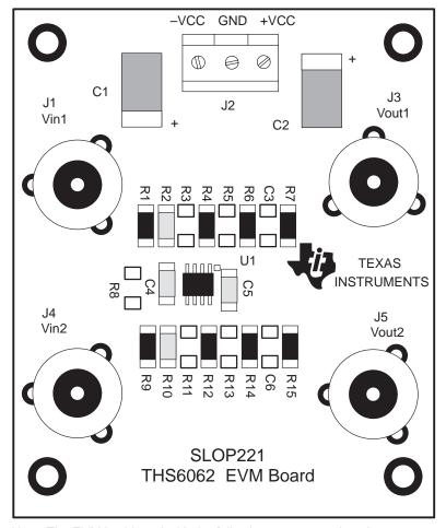
Note: The EVM is shipped with the following component locations empty: C3, C6, R3, R5, R8, R11, R13
