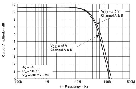
Figure 1–5. THS6062 EVM Frequency Response with Gain = –3
