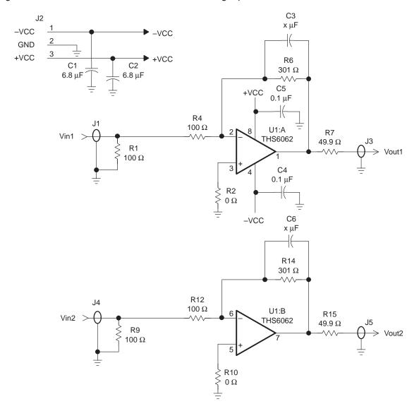
The gain of the EVM can easily be changed to support a particular application by simply changing the ratio of resistors R6 and R4 (channel 1) and R14 and R12 (channel 2) as described in the following equation:
